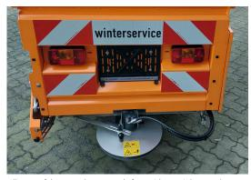
All parts of the spreader are made from either stainless steel or lacquered with varnish in corrosion-class C5.
